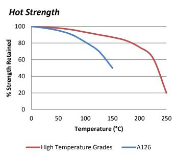
"Hot strength" Breakaway strength on M10 Zinc plated bolts according to ISO 10964. Cured at 23°C for 24 hours then conditioned for 30 minutes at testing temperature.
