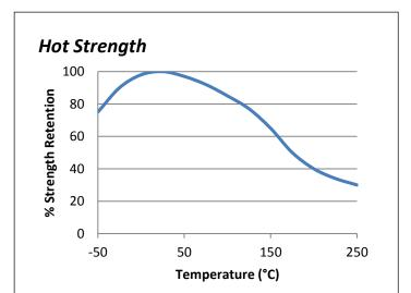
"Hot strength" shear strength tests performed on mild steel. Initially cured at room temperature and then post-cured at 150°C for 2 hours.
