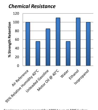
Specimens were immersed for 1000 hours at  $22^{\circ}$ C (unless otherwise stated).
