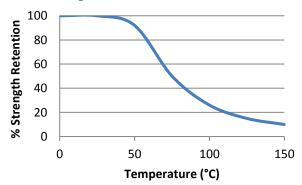
"Hot strength" shear strength tests performed on mild steel. Fully cured specimens conditioned to pull temperature for 30 minutes before testing at temperature. ET5364 can withstand higher temperatures for brief periods (such as for paint baking and wave soldering processes) providing the joint is not unduly stressed. The minimum temperature the cured adhesive can be exposed to is -40°C (-40°F) depending on the materials being bonded.
