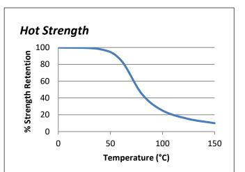
ET5381 can withstand higher temperatures for brief periods (such as for paint baking and wave soldering processes) providing the joint is not unduly stressed. The minimum temperature the cured adhesive can be exposed to is -40°C (-40°F) depending on the materials being bonded.
