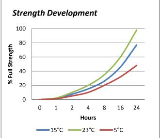
Graph shows typical strength development of bonded components. Increasing the curing temperature will result in a faster cure, colder conditions may slow cure slightly, but this is less marked than with most other epoxies.
