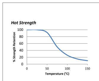
"Hot strength" shear strength tests performed on mild steel. Fully cured specimens conditioned to pull temperature for 30 minutes before testing at temperature.
