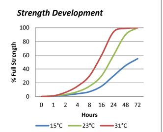
Graph shows typical strength development of bonded components. An increase of 8°C in temperature will halve the cure time. Lower temperatures will result in a slower cure time.
