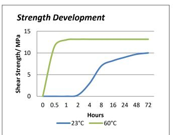
Graph shows typical strength development of bonded aluminium components. Curing at 60°C improves the crosslinking and results in higher final strength values. Lower temperatures will result in a slower cure.
