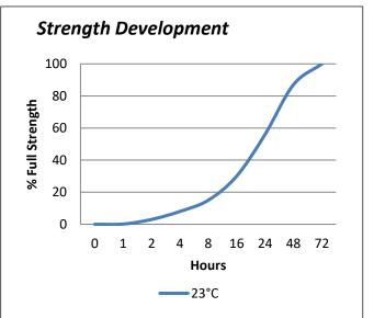
Graph shows typical strength development of bonded components at 23°C. Curing at higher or lower temperatures may affect cure speed.
